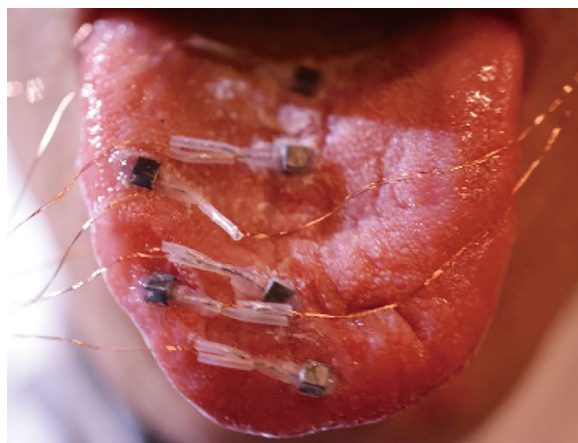
Using a magnetic measuring device to measure tongue movement
