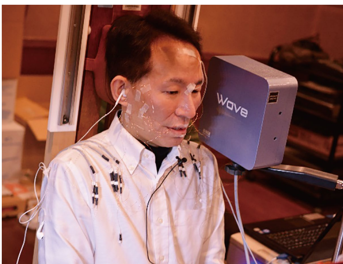
Using a magnetic measuring device to measure tongue movement
